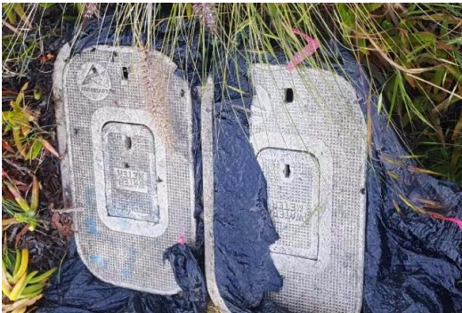
Water meter boxes
